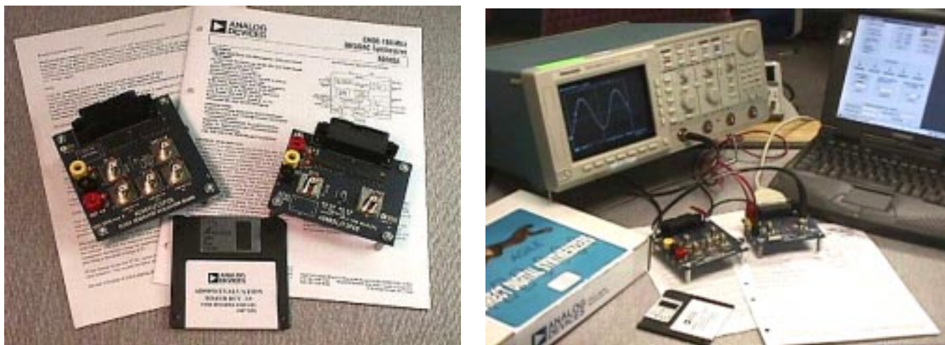
Figure 12-1. Typical Evaluation Kits for DDS Products
