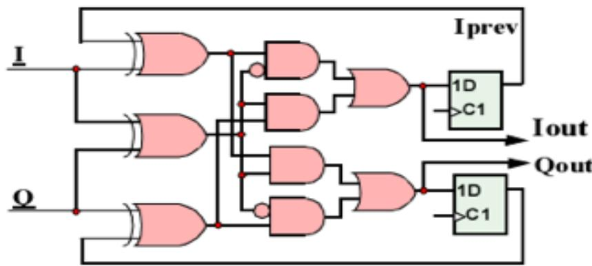
$$I_{out} = \overline{I} \oplus \overline{Q} (I \oplus I_{prev} + (I \oplus Q)(Q \oplus Q_{prev}))$$
