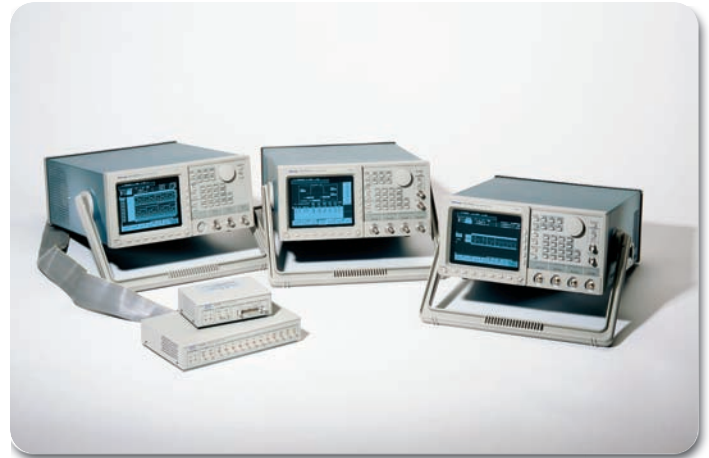
► Figure 47. The DG2020A pattern generator uses an external signal interface "pod."
