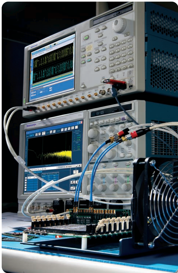
▶ Figure 1. Most measurements require a solution made up of a signal generator paired with an acquisition instrument. Triggering connectivity simplifies capturing of the DUT output signal.
